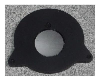
The external reference mirror is supplied uncalibrated in which case the user should generate the reflectance values by comparison with their working standard. Reflectance values should be determined for each of the aperture settings 15 mrad and above that are used for measurements.
