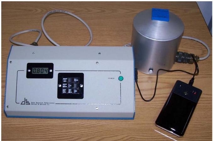
To make the D&S Solar Spectrum Reflectometer Model SSR-ER portable, an optional battery pack can be attached. The battery pack comes with its own rechargeable battery, charging system, and carrying case.
